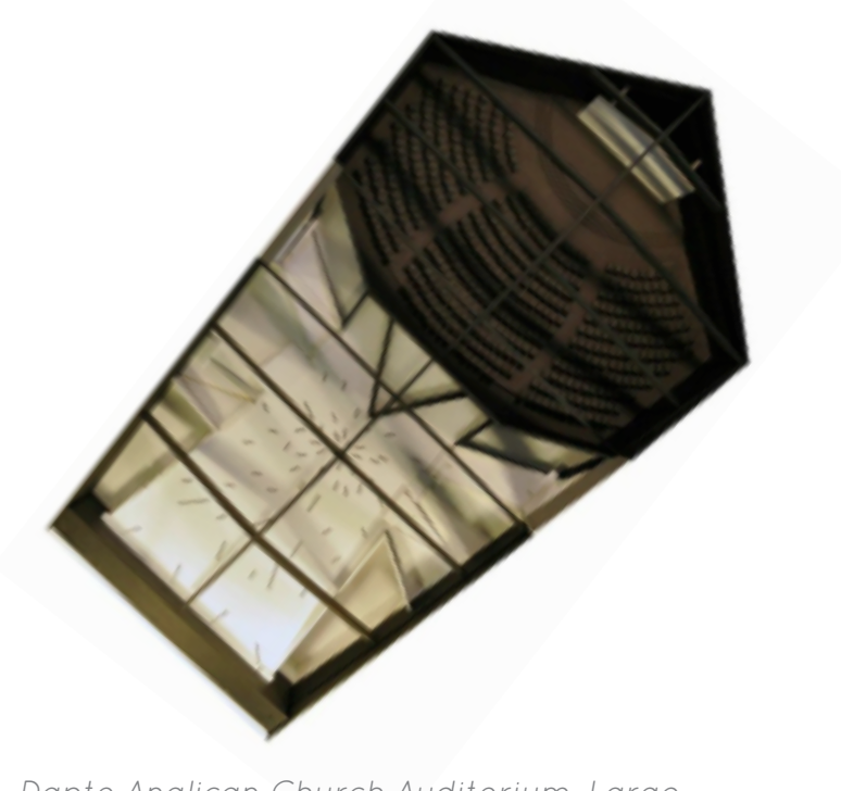
Dapto Anglican Church Auditorium, Large scale model, showing the roof trusses and a lighting option reflecting people densities, Silvester Fuller, 2011.
